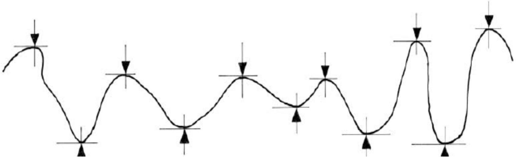
Note: The upper arrows indicate the levels of available maximum quantity of water and the lower arrows indicate the levels of available minimum quantity of water.
